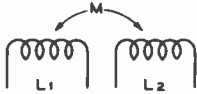
Figure 18. MUTUAL INDUCTANCE. The quantity M represents the mutual inductance between the two coils L 1 and L 2 .
