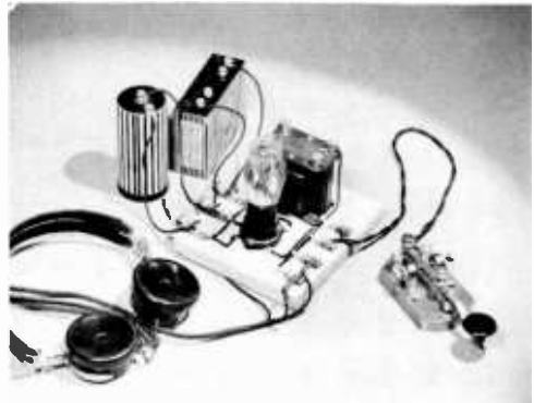
Figure 7. THE CIRCUIT OF FIGURE 6 IS USED IN THIS BATTERY-OPERATED CODE PRACTICE OSCILLATOR.
