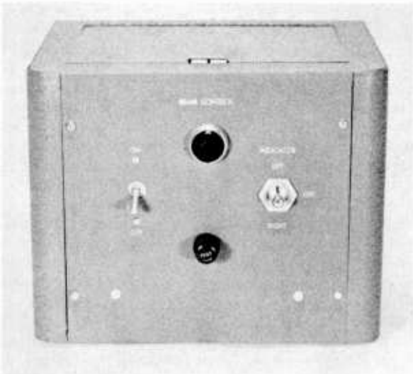
Figure 30. CONTROL BOX FOR THE ANTENNA ROTATION SYSTEM.
